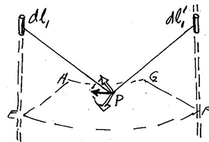
(2) The contributions to the field at  $P$  from equal, symmetrically located wire elements  $dl_2$  and  $dl'_2$  also combine to form a resultant in the circumferential direction. Here the individual vectors are out of the plane, and the geometry is a little harder to visualize.
