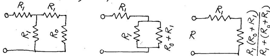
$$R = R_1 + \frac{R_1(R_0 + R_1)}{R_1 + (R_0 + R_1)}$$
