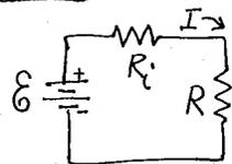
Let  $P$  = power dissipated in resistor  $R$
