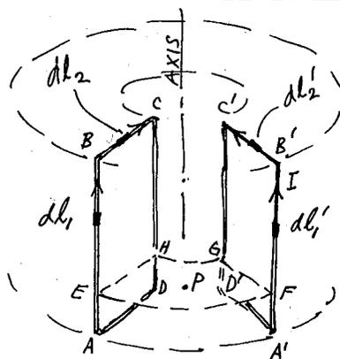
(1) The contributions to the field at  $P$  from equal, symmetrically located wire elements  $dl_1$  and  $dl'_1$  combine to form a resultant in the circumferential direction. (Note that each vector lies in the plane  $EFGH$ .)
