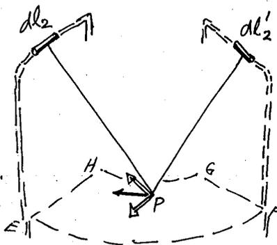
Since the two rectangular turns can be entirely decomposed into such elements, and the entire coil can be decomposed into such pairs of turns, it follows that the total field at  $P$  must be circumferential.
