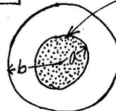
Current  $I$  is uniformly distributed over the cross-section of the inner conductor, and returns in outer conductor whose thickness we neglect.
