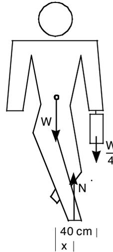
Next, redraw Fig. 1.13 with the foot 8 cm across the midline. The normal force is now  $(5/4)W = 1.25W$ . The weight of the leg ( $W/7$ ) still acts  $10/18$  of the way along the leg or  $10/18$  of the horizontal distance from greater trochanter to the foot.  $(10/18)(18 + 8) = 14.4$  cm. Assume  $\mathbf{F}$  has not changed direction and that the horizontal component still exerts negligible torque around the point in the head of the femur.
