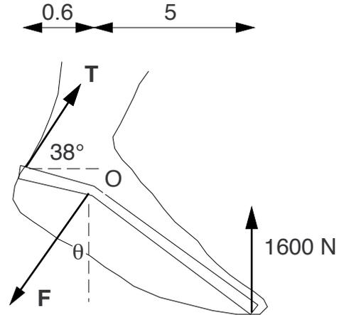
$$\begin{aligned}F \sin \theta &= T \cos 38^\circ = 1.71 \times 10^4 \\ F &= [(1.5 \times 10^4)^2 + (1.71 \times 10^4)^2]^{1/2} = 2.3 \times 10^4 \text{ N} \\ \theta &= \tan^{-1}(1.71 \times 10^4 / 1.5 \times 10^4) = 49^\circ\end{aligned}$$
