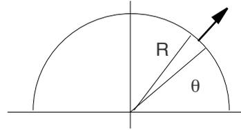
We can get the same answer by direct integration of the force exerted on the hemi-cylinder by the gas inside. Consider the strip of length  $L$  and width  $Rd\theta$ . The force is pressure times area:  $d\mathbf{F} = pdS = pRL d\theta$ .
