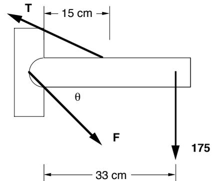
**1.8** If torques are taken about O, the slight vertical displacement of the point of application of  $T$  can be neglected.
