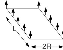
By the third law, the reaction to this is the force on the hemi-cylinder. This force is the same whether it is exerted by a flat plate or by another hemi-cylinder.
